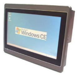
PTH-1070A touch panel computers provides an open HMI platform for most automation applications. Equipped with Marvell PXA 270 RISC processor and 5.7" or 7" TFT panel with touch screen, PTH-1070A provides fan less solution with up to 800 x 600 TFT
