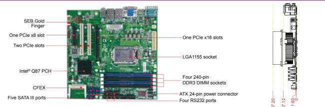
RUBY-D720VG2AR is based on Intel® Q87 chipset and desktop processor sku like Core Intel Core 4th Gen. Build with PCI and PCI Express expensions, it is suitable for Medical, Industrial automation, and digital signage ap-plications.
