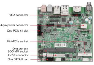
NANO-5050 adopts latest Intel<sup>®</sup> Atom<sup>™</sup> D2550/ N2800/ N2600 CPU and NM10 chipset which is for the low power compact size system. The new archi-tecture integrates the 3D graphics engine and memory controller. It's suitable for Medical and Networking applications.
