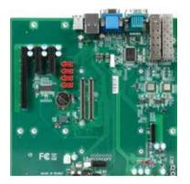
PCOM-C609 is Portwell's first carrier board designed to support 10 Gigabit Ethernet function. Specifically, PCOM-C609 is a microATX form factor carrier board supporting 10GbE, USB 3.0, PCIe, HDMI, VGA, SATA and TPM interfaces. PCOM-C609 is designed with COM Express Type VI row connectors, and is suitable for evaluation and testing with Portwell's Type VI COM Express modules.
