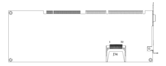
Figure 2-2 ROBO-8612VGA Connector Location (Solder Side)
