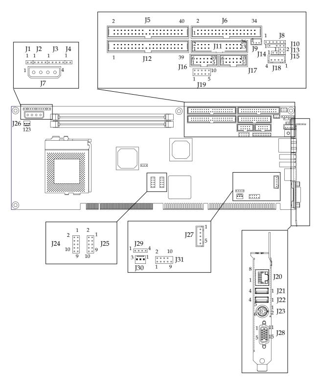
Figure 2-2 ROBO-8612VGA Connector Location (Component Side)
