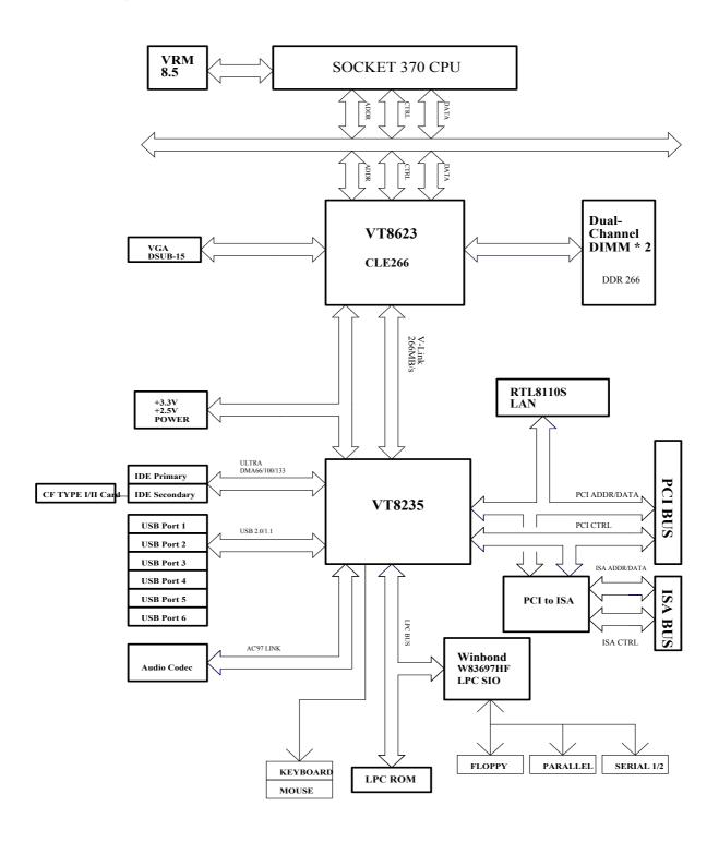
ROBO-8612VGA System Block Diagram
