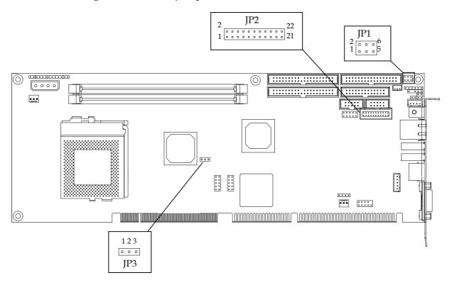
Figure. 2-1 ROBO-8612VGA Jumper Location
