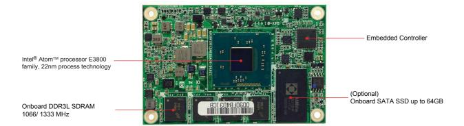
PCOM-BA00 is the latest Mini COM Express by 84mm x 55mm with Intel Bay Trail E3800 series SoC supports PCI Express, dual display, NANDrive storage features.
