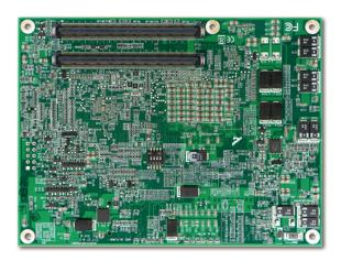
The basic PCOM-B635VG COM Express module supports up to 16GB ECC DDR3L 133/1600 MT/s SDRAM on two 204-pin SO-DIMM sockets making it faster than its predecessor. Its expansion interface supports one PCI Express x16 Gen3 (8.0GT/s) with three controllers integrated into processor for enhanced video performance and enhance capabilities to be configurable to 2 x8-lane or 1 x8-land and 2 x4-lane PCI Express ports.
