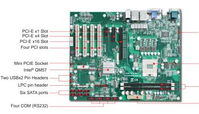
Built with latest mobile Intel® QM57 Express chipset which supports Intel® Core™ i5/ i7 processor, RUBY-M710VG2AR based industrial ATX motherboard is the ideal solution for Green PC and can be adopted in POS, medical, gaming, lottery, digital signage, surveillance security monitoring and kiosk.
