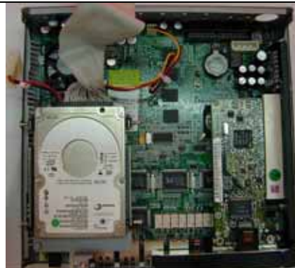
(Fig. 2-17). Add 2.5' HDD and Connect IDE Cable and power cable to system
