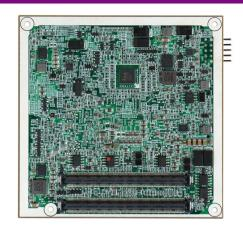
PCOM-B631VG can provide good computing by Dual Core processor with lower power consumption comparing with Haswell 2-chip platform. Multi-display support, such as LVDS/eDP/DP/VGA, is convenient to meet customer's display output requirement.
